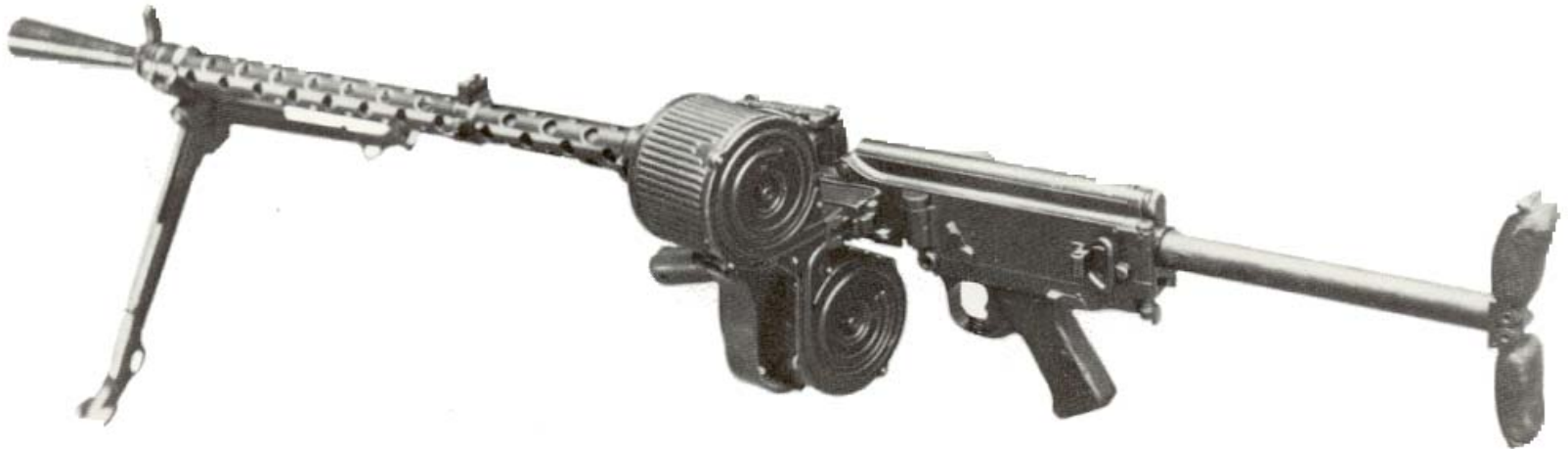
The Dreyse MG13, an alteration to the old water-cooled MG10 used in small numbers in World War 1. The conversion was executed c.1933-4 to supply the Wehrmacht with a suitable light machine-gun pending the development and issue of the MG34.
