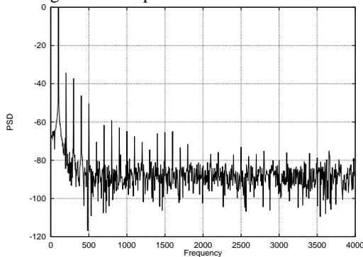
Figure 1. Typical interference spectrum of an incandescent lamp.
