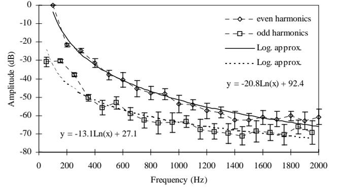
Figure 5. Average amplitude of each interference component.
