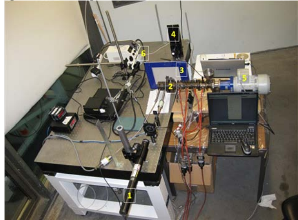
Figure 3 – Rheo-optical slit die coupled to SALS set-up and mini-extrusion line.
