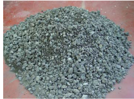
Figure 1. Portuguese processed steel slag (ISAC).
