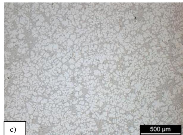
Figure 6: Microstructures of AlSi9Cu3 alloys obtained: a) Without US; b) with 200 W of US; c) with 600 W of US.
