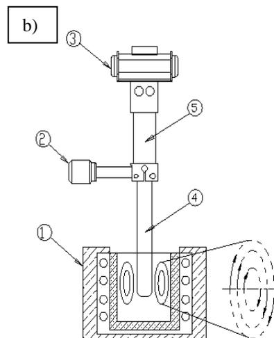
Figure 1: a) Degassing laboratorial unit; b) components of unit of degassing: (1) furnace, (2) ultrasonic transducer, (3) low frequency mechanical vibrator, (4) radiator, (5) helicoids interface.
