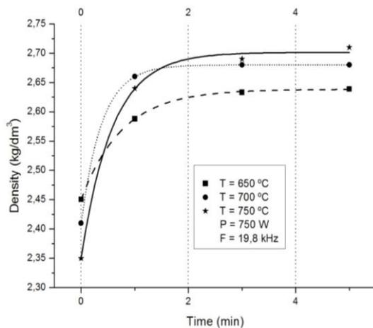
Figure 4: Density of the AlSi9Cu3 alloy as a function of melt temperature and processing time, for 19.8 kHz resonant frequency and 750W electric power.
