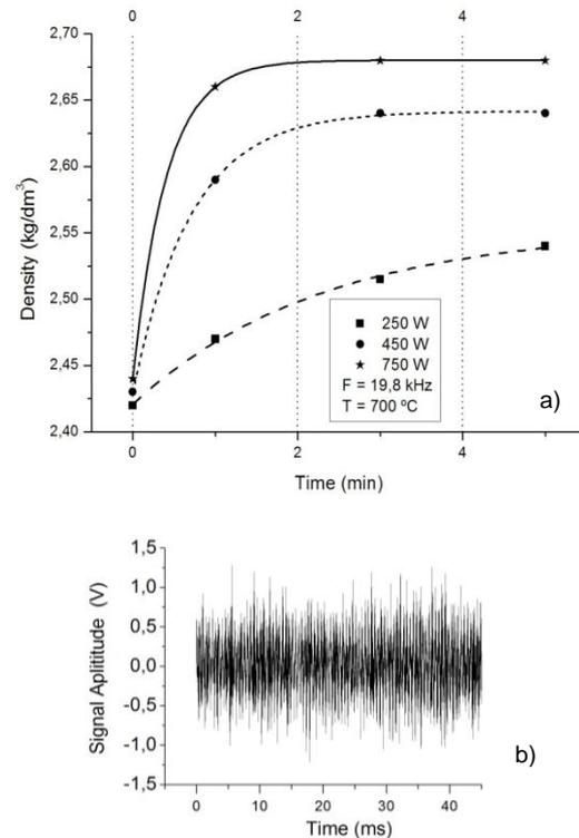
Figure 3: a) Density of the AlSi9Cu3 alloy as a function of electric power and processing time, for 700°C melt temperature and 19800±100 Hz resonant frequency; b) acoustic waves in the molten metal for 750 W electric energy.
