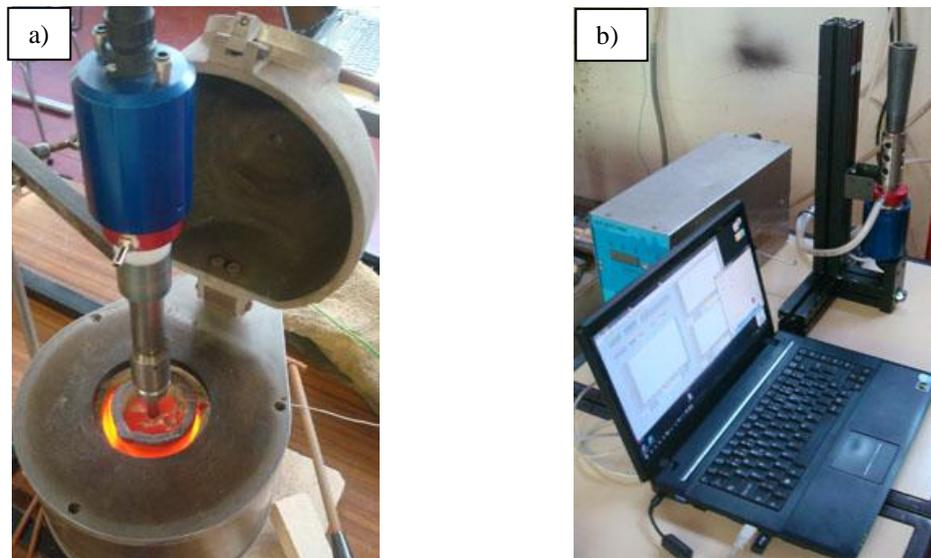
Figure 2: Ultrasonic laboratorial unit: a) isothermal processing by vibration of melt; b) by ultrasonic vibration applied to the mould.
