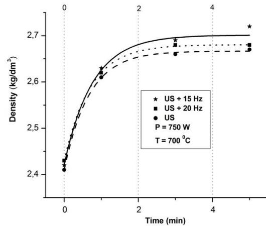
Figure 5: Density of the RPT samples and degassing efficiency of the AlSi9Cu3 alloy as a function of mechanical vibration frequency and processing time, for 700°C melt temperature.
