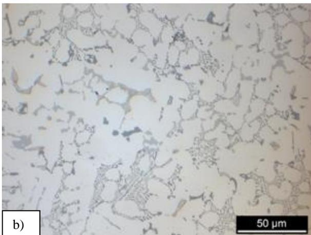
Figure 7: Microstructure of a AlSi9Cu3 sample ultrasonically treated at 600 W during cooling: a) 50 X; b) 500 x.
