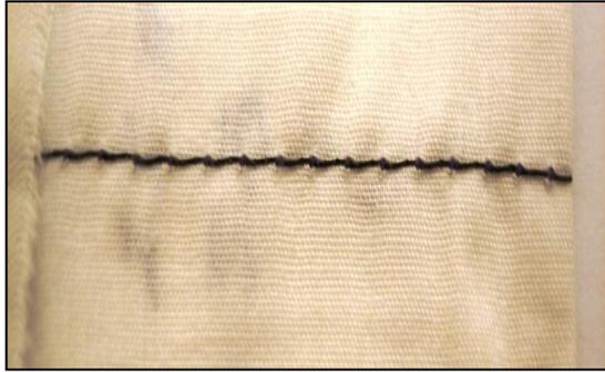
Figure 7: Seam made with PP/4%CNT monofilament
