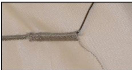
Figure 8: Attachment of TPU/ 4% CNT monofilament
