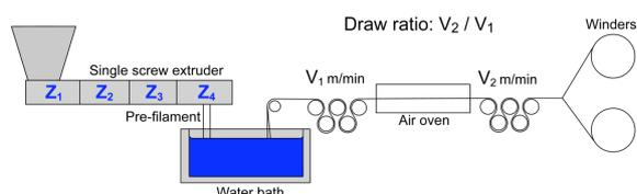
Figure 2: Equipment setup for monofilament extrusion and drawing
