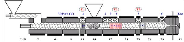
Figure 1: Extruder layout used for the preparation of the CPC composites
