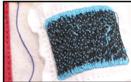
Figure 10: Fabric surface obtained using the monofilament as bobbin thread on a lockstitch sewing machine
