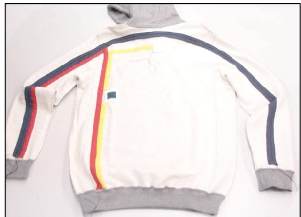
Figure 11: Prototype garment produced with sensing monofilaments incorporated
