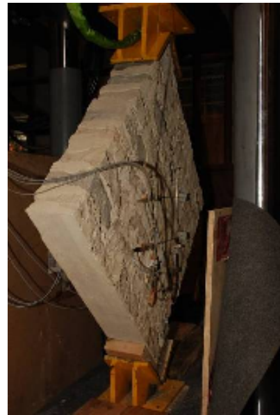
Figure 4: Test setups for specimens in diagonal compression tests
