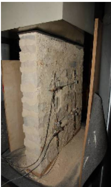
Figure 3: Test setups for specimens in axial compression tests
