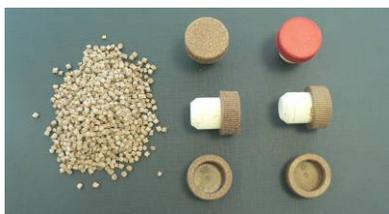
Figure 3: Bio-based cork pellets and scale-up of the final solution with application as biodegradable cap.
