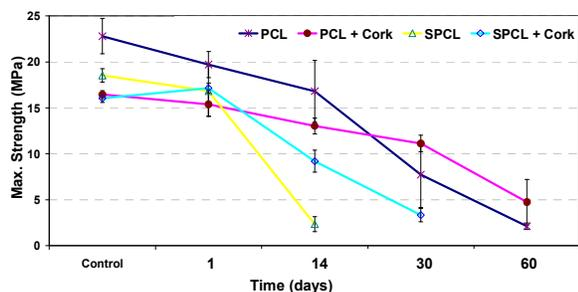
Figure 1: Tensile strength properties of the bio-composites after soil degradation tests during 60 days.
