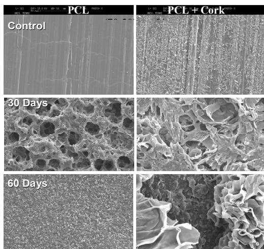
Figure 2: Morphology after soil the degradation tests.
