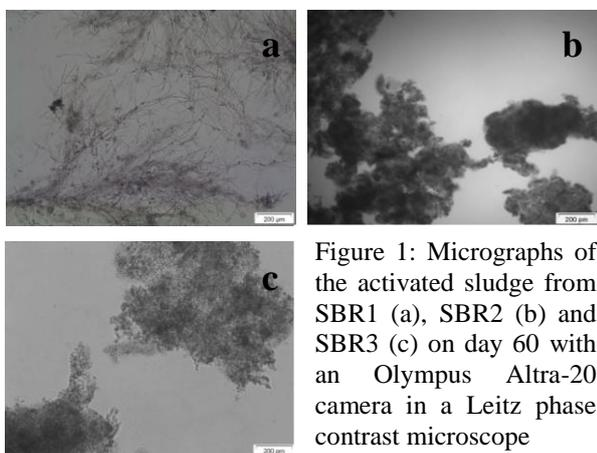
Figure 1: Micrographs of the activated sludge from SBR1 (a), SBR2 (b) and SBR3 (c) on day 60 with an Olympus Altra-20 camera in a Leitz phase contrast microscope
