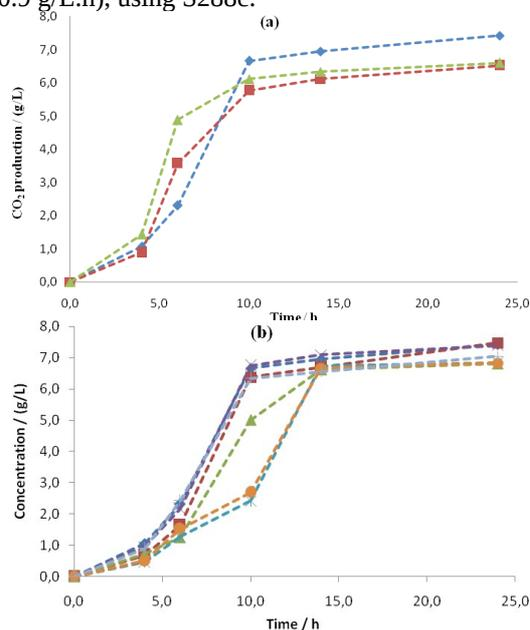
Figure 1: CO<sub>2</sub> production during fermentation in: (a) YPDb control, using: (♦) S288c, (■) CA11 and (▲) PE-2; and (b) YPDb using S288c in: (♦) control, (■) ethanol, (▲) 1-butanol, (×) isopropanol, (+) 2-methyl-2-butanol, (\*) 2-furaldehyde, and (●) 5-HMF.
