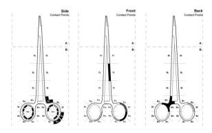
Figure 3. Ergonomic evaluation in a needle holder
