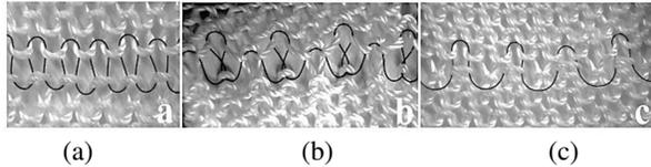
Figure 1: Knitted structures showing stitch loop (a), tuck loop (b) and miss loop (c).
