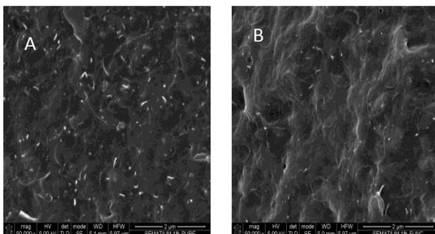
**Figure 2** – SEM images for pure A) and functionalized B) 1% CNT nanocomposites.
