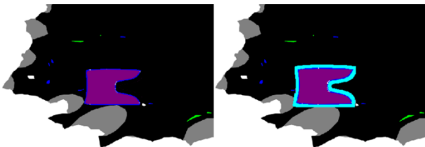
Figure 4: Intersection between the offset of a piece and the non-usable region of the hide
