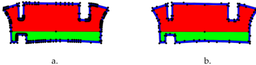
Figure 3: Representation of a piece before (a.) and after (b.) the vertex removal procedure
