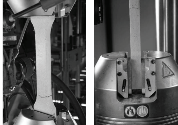
Figure 1: Test-setup to assess tensile stress-strain behavior.
