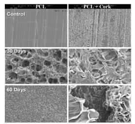
Figure 2: Morphology after soil the degradation tests.
