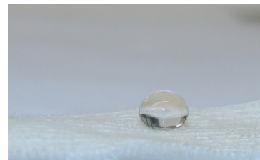
Figure 3 – Water drop on the sample PLA fabric nanocoating with superhydrophobic properties, " Lotus effect "
