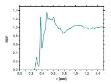
**Figure 2.** Pair correlation function of C-C in polyethylene
