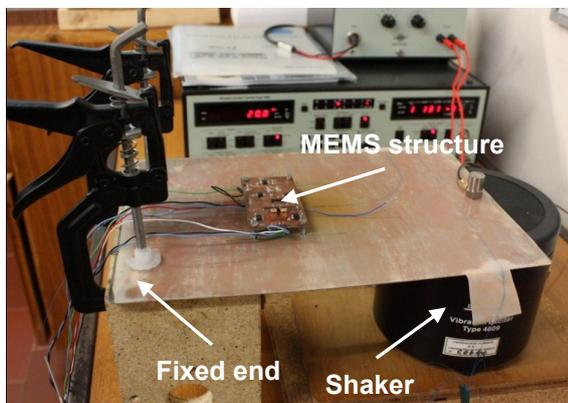
Figure 4: Experimental setup with the microstructure and the readout circuit mounted on a movable platform
