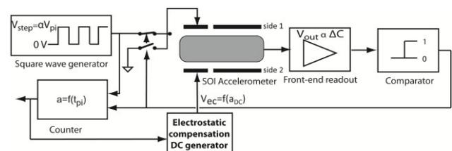
Figure 1: Microaccelerometer block diagram
