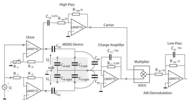
Figure 3: Displacement detection circuit with charge amplifier and AM demodulation stage
