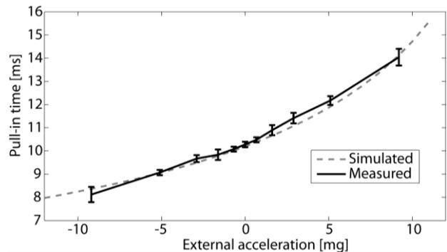
Figure 5: Accelerometer pull-in time response to small external accelerations.
