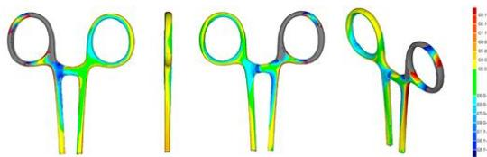
Figure 2: Shape analysis of a needle holder
