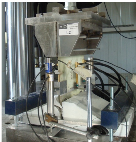
Figure 2: Experimental setup for the pull-out tests.
